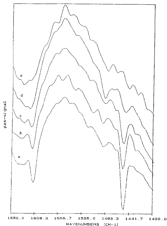
Fig. 2. FT-IR/PA spectra of pyridine desorbed from silica gel 60 containing 9 wt.% Cu, in the (1650–1400 \text{cm}^{-1} ) range, at the following temperatures: spectrum a, 373 K; spectrum b, 410 K; spectrum c, 450 K; spectrum d, 523 K; spectrum e, 663 K.
